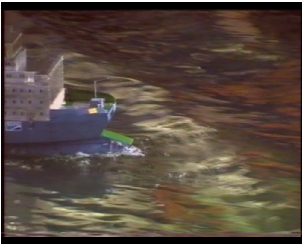
Bow ramp has opened and the water floods the car deck giving a heel angle of 25 degrees within 10 seconds (one minuter in full scale)
