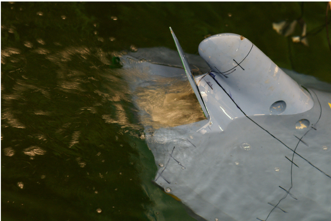
Ship model in heel angle 150-160 degrees. Due to scale effects in air compressibility air was ejected from a calibrated valve at the stern of the model.
