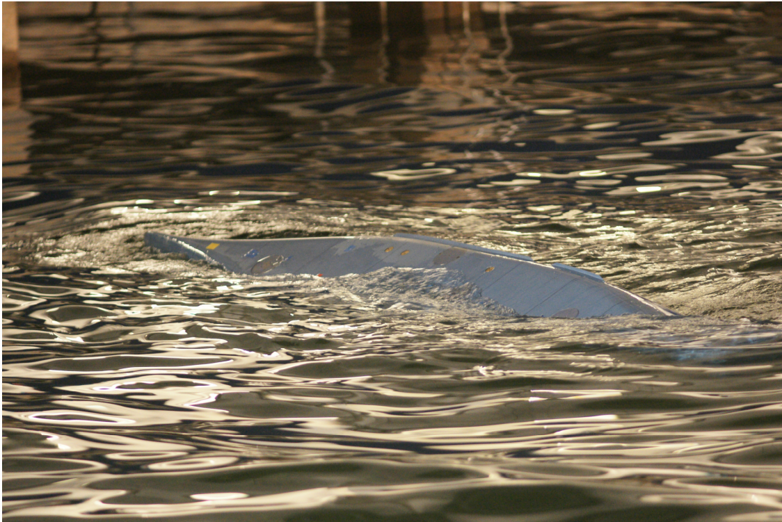
Ship model in heel angle 150-160 degrees. Due to scale effects in air compressibility air was ejected from a calibrated valve at the stern of the model.
