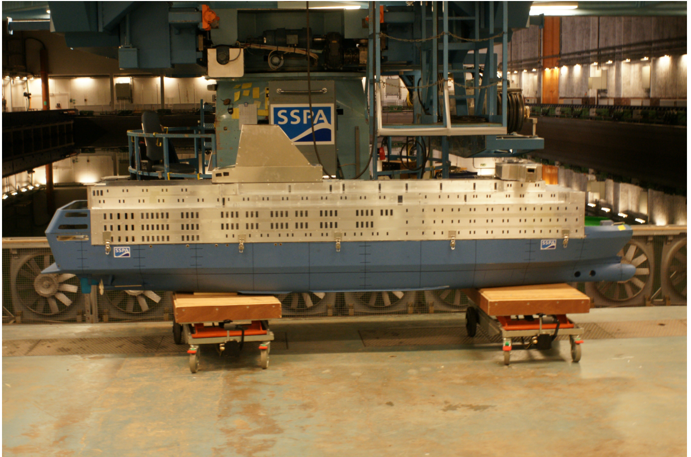
The ship model of MS Estonia. In the background the Maritime Dynamics Laboratory with the wind battery mounted on the carriage.
