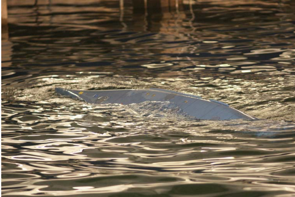
Fig. 34. Ship model in heel angle 150-160 degrees. Due to scale effects in air compressibility air was ejected from a calibrated valve at the stern of the model.
