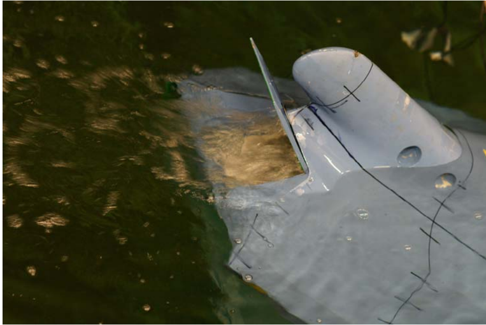
Fig. 35. Final phase of the foundering. The stern has rested at the bottom of the basin and air is escaping from the car deck. Due to practical reasons the ramp was forced open during the tests, but would have been closed by gravity by now.
