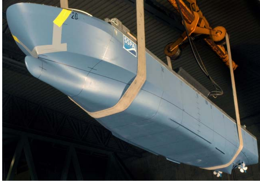
Fig. 9. Photo of model of MV Estonia used for the manoeuvring and sea keeping tests.
