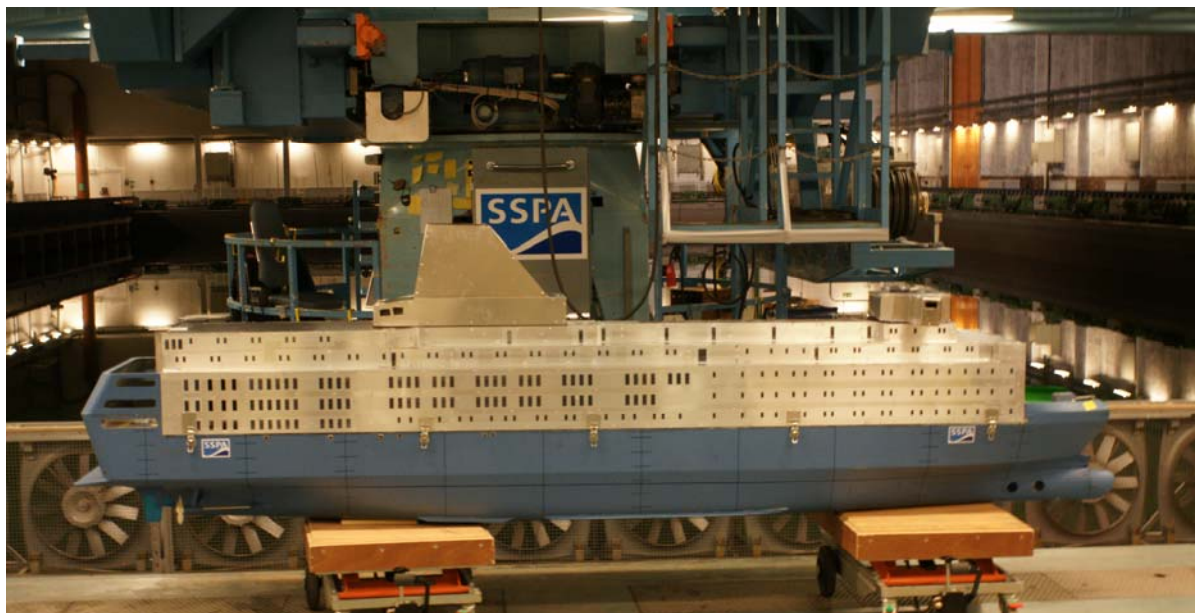
Fig. 33. The ship model used for the foundering tests. In the background the SSPA’s Maritime Dynamics Laboratory with the wind battery is shown.
