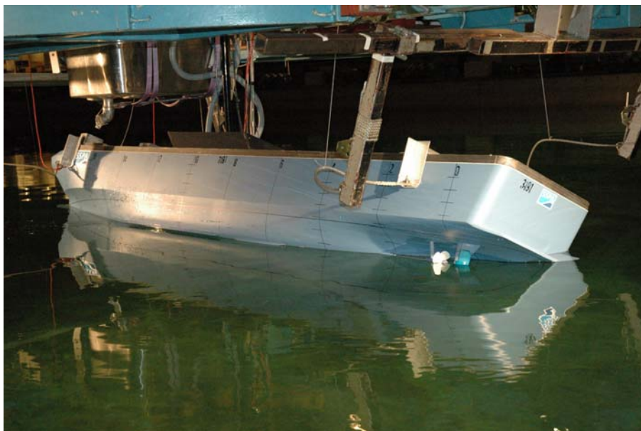
Fig. 11. Model set-up for turning tests. At 25 degrees heel angle the port shaft is in the waterline and the port rudder half out of water, which significantly influences the behaviour of the ship.
