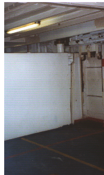
Figure 3.21.4 - The movable 'watertight' bulkhead at the side
