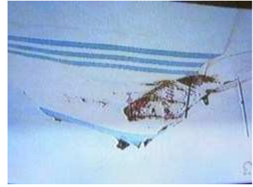
Fig.1.1.6 - The buckle in the 'Estonia' visor - what caused it?
