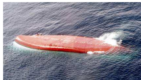
Figure 1.50.1 – Ferry floating after capsizing without 'watertight' deckhouse
