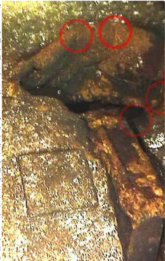
Fig. 3.8.2 - SB side lug in its recess. Recess top severely damaged (Source International Fact Group)
