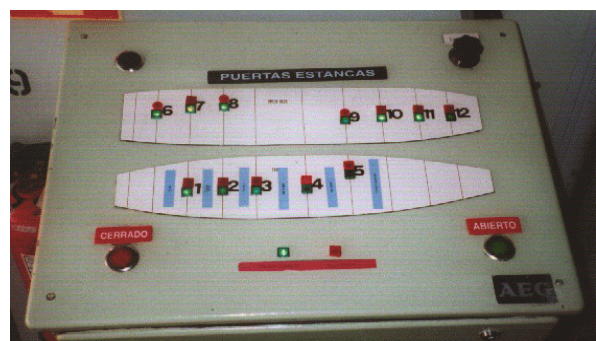
Figure 1.23.1 - Incorrect watertight door control panel - year 2002
