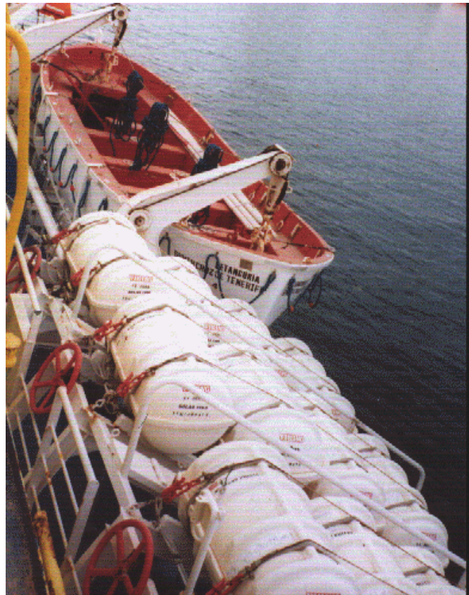
Figure 1.33.1 - Illegal life raft arrangement - year 2002!
