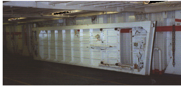
Figure 3.21.2 - Movable 'watertight door/bulkhead' in the side of the superstructure
