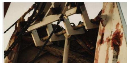
Fig. 3.8.3 - Visor just after salvage - manual hooks
